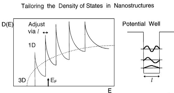
Fig. 3. Schematic of how confinement to a nanostructure can be used to modify the density of states at the Fermi level  $E_F$ . Quantum well states lead to maxima in the density of states. These can be swept through  $E_F$  by varying the width  $l$  of the quantum well (see Eq. (1)).
