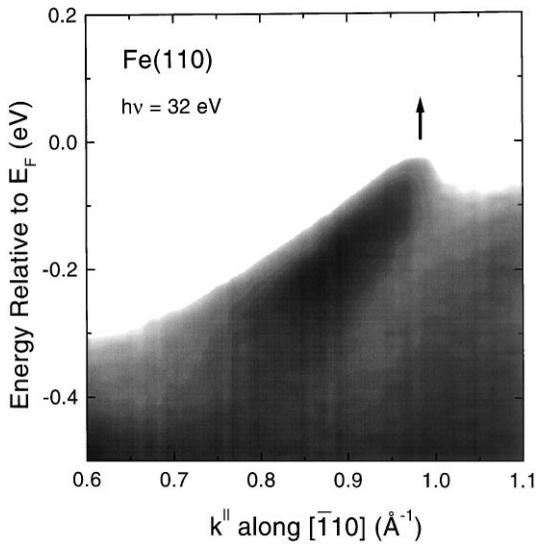
Fig. 5. Photoemission data of the Fermi level crossing of the majority spin s, p-band in Fe(1 1 0) along the  $[\bar{1} 1 0]$  azimuth.
