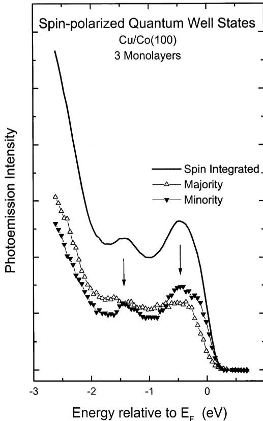
Fig. 8. Spin-resolved photoemission spectra of short-period quantum well states in Cu/Co(100) that are derived from the neck of the Cu Fermi surface ( $h\nu = 77$  eV,  $\theta = 11^\circ$  along  $[0\ 1\ 1]$ ). Minority spins are reflected at the interface and confined to the Cu layer, giving rise to peaks for discrete quantum well states (arrows). Majority spins are transmitted and preserve the continuous, bulk-like spectrum.
