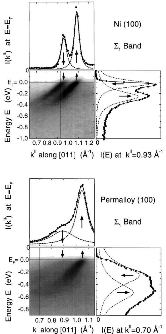
Fig. 6. Photoemission from the Fermi level crossing of the  $\Sigma_1$  s, p-band in Ni and permalloy ( $\text{Ni}_{0.8}\text{Fe}_{0.2}$ ), together with cuts along constant  $E$  and  $k$ . Lorentzian fits provide lifetimes and scattering lengths (Eqs. (8)–(10)). Majority and minority spins are denoted by up and down arrows.
