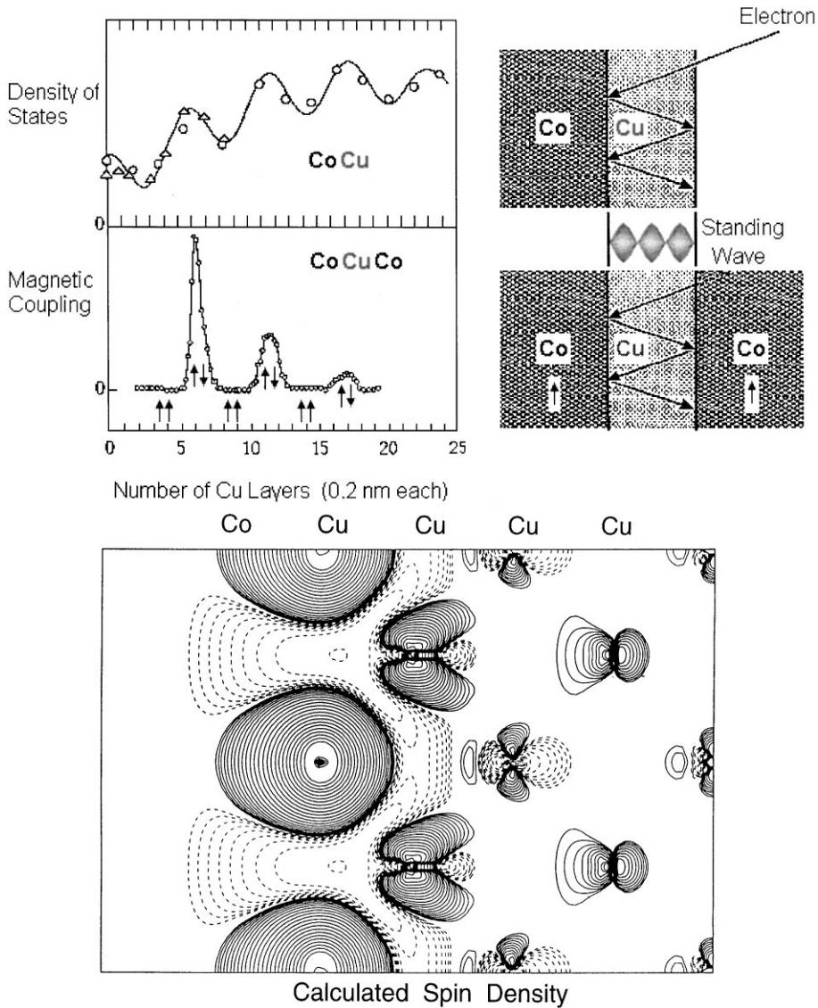
Fig. 7. Oscillatory magnetic coupling in Co/Cu/Co(100) driven by quantum well states at  $E_F$ . The long-period oscillations observed via the Kerr effect (from Qiu et al. [62]) are synchronous with the density of states maxima [56,57] created by quantum well states at the belly of the Cu Fermi surface. A calculation of the spin density wave introduced by all quantum well states is given on the bottom (from Wu and Freeman [64]).
