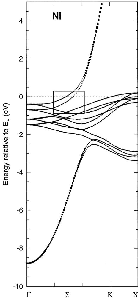
Fig. 1. Empirical  $E(\mathbf{k})$  band dispersions of Ni along the  $[1\ 1\ 0]$  direction ( $\Sigma$  line). Bands with more than 50% s, p-character are shown in bold. A parabolic s, p-band crosses a set of flat d-bands and hybridizes with them, forming an avoided crossing. Carriers located at the Fermi level crossing of this hybrid band (box) are likely to dominate magnetic transport properties.
