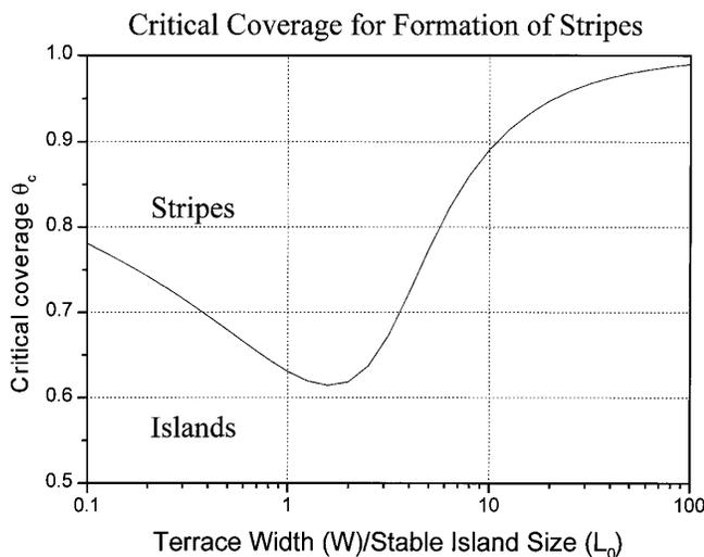
FIG. 4. The upper limit of critical coverage  $\theta_c$ , for transition from rough growth fronts (platelets) to smooth growth fronts (stripes), as a function of the ratio of the width of substrate terrace and the stable size of a single island ( $W/L_0$ ).
