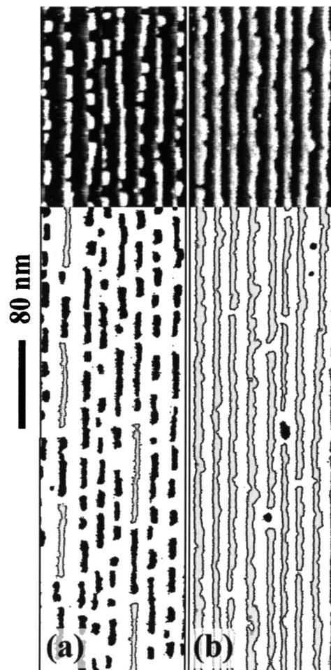
FIG. 3. STM images of  $\text{CaF}_2$  on stepped Si(111), showing the transition from platelets to stripes. The two samples are prepared under the same conditions, except for the coverage, 0.23 ML in (a) and 0.40 ML in (b). Top portion of the images shows STM topography, bottom is color coded—platelets [black, dominant in (a)] and stripes [gray, longer than 80 nm, dominant in (b)].
