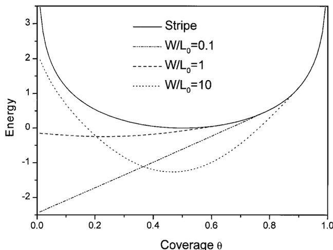
FIG. 2. The strain energy per unit area of the stripe configuration (the solid line) and of the island configuration (the broken lines) for different values of  $W/L_0$ , i.e., the ratio of the substrate terrace width ( $W$ ) and the size of stable isolated island ( $L_0$ ). The island configuration always has lower strain energy than the stripe configuration at the beginning of the growth (low coverage) for any  $W/L_0$ .
