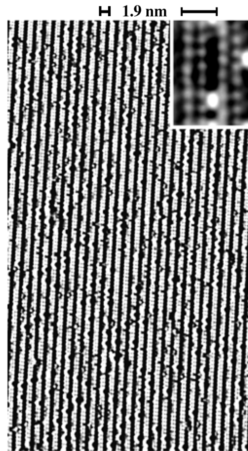
FIG. 3. STM images of the Si(557)-Au surface revealing a one-dimensional structure with two nearly equivalent chains of atoms in the unit cell (inset). The overview shows the derivative of the topography, the inset the topography itself. The [\bar{1}\bar{1}2] direction (downhill) is to the right.
