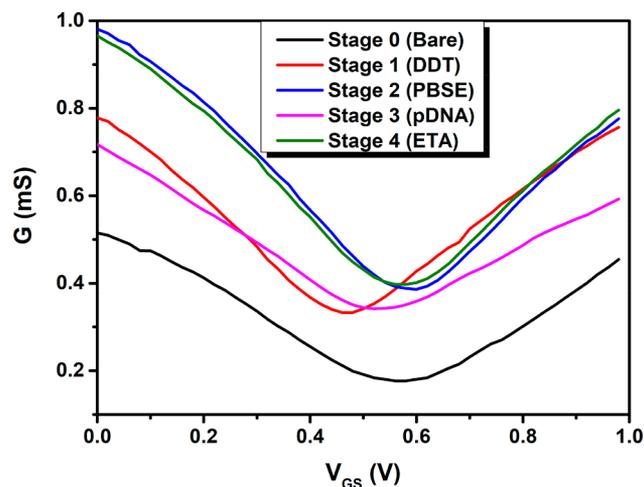
**Figure 2.** Characteristic transfer curves after each stage of the EGFET channel functionalization.
