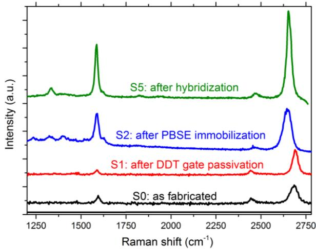
**Figure S4** – Characteristic room temperature Raman spectra of the graphene channel of the transistor after stages 0, 1, 2, and 5 of the functionalization/biorecognition process. Spectra S0 and S1 were obtained with 532 nm laser excitation line and S2 and S5 with 633 nm laser line.
