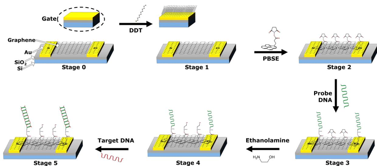
**Figure S1.** Schematic view of the stages of the biosensor development: Stage 0: as-fabricated graphene transistor; Stage 1: DDT gate passivation; Stage 2: immobilization of the linker (PBSE); Stage 3: functionalization with probe DNA; Stage 4: blocking with ethanolamine; Stage 5: biorecognition.
