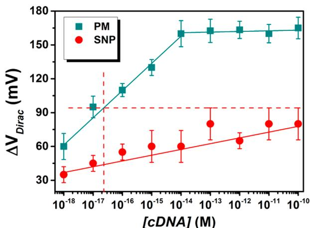
**Figure 4.** Calibration curves for the bio-FET sensor. Green squares refer to target DNA fully complementary to the probe and red circles to SNP target. The error bars are standard deviations of measurement with five different devices.
