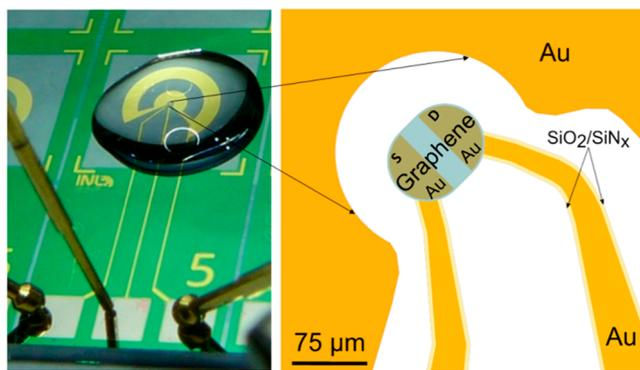
**Figure 1.** (left) Optical image of one transistor chip under measurement; (right) drawing of the transistor zoomed-in channel region, showing source (S), drain (D), gate (partial view), and Au contact lines with SiO<sub>2</sub>/SiN<sub>x</sub> passivation layer.
