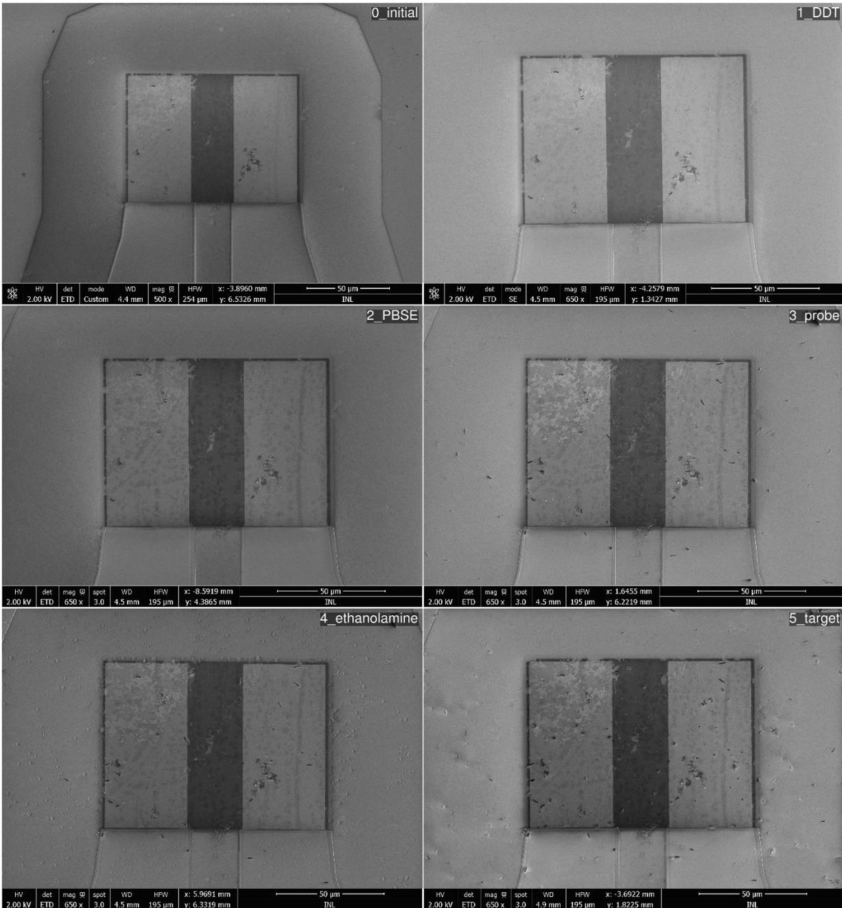
**Figure S8** – SEM images of the graphene channel (dark area) of one transistor, in between source and drain Au contacts (clear areas), taken after each of the stages of the biosensor development (see main text and Figure S1). Note that the graphene overlaps the Au S-D contacts, exceeding a few micrometers the Au contact (dark edge). Note: the rectangular source and drain contacts in the images above are slightly different in shape from those shown in the main text (semi-circular).
