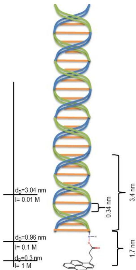
**Figure S7.** Schematic illustration of a DNA double helix bound to a PBSE linker that links to graphene. Left scale shows Debye length,  $d_D$ , as a function of electrolyte ionic strength calculated by Debye-Hückel theory. Right scale shows characteristic molecular lengths.
